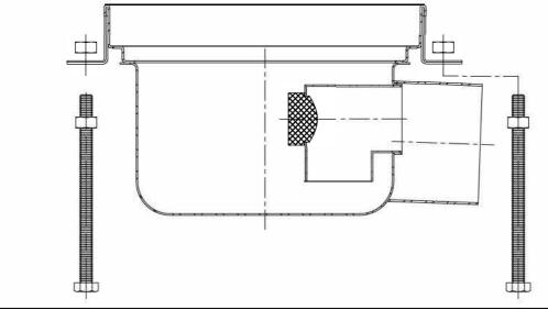
\*IN CASE APPLICATION OF ADJUSTING FEET IS REQUIRED, AS A FIRST STEP, THE BOLTS AND NUTS ARE FIXED ON THE BODY AS SHOWN BELOW.
